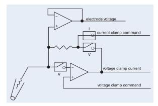
**Simplified CV-7B diagram.** The CV-7B headstage contains both resistor feedback voltage-following circuitry for true current-clamp operation, and voltage-to-current circuitry for voltage-clamp operation.
