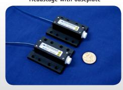
The small profile of the miniaturized HS-9A and VG-9A headstages makes it easy to incorporate them into an electrophysiology set up. The dovetail design integrates with a baseplate for easy attachment to micromanipulators.
