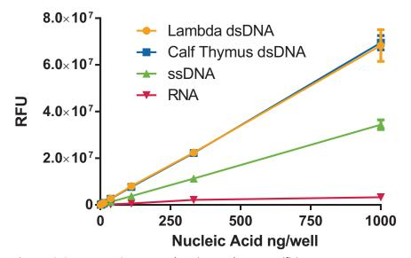
Figure 1-2: SpectraMax Quant AccuBlue HiRange dsDNA specificity assay
