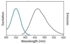
Figure 1-1: SpectraMax Quant AccuBlue HiRange dsDNA assay dye fluorescent excitation and emission spectra
