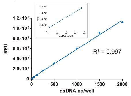
**Figure 4-1: SpectraMax Quant AccuBlue HiRange dsDNA assay standard curve** Linearity of the SpectraMax Quant AccuBlue HiRange dsDNA assay between 2 ng and 2000 ng per well in a 96-well microplate assay with excitation = 350 nm and emission = 460 nm. The inset shows the lower portion of the curve.
