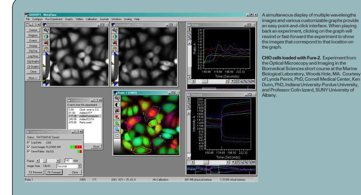
When acquiring from video sources, MetaFluor can average up to 256 images per time point, significantly reducing random image noise. Background subtraction is also used to improve accuracy by correcting for stray light, camera noise and auto-fluorescence.
