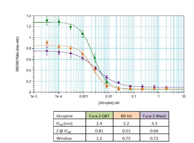
Figure 6. The FlexStation3 Instrument was used to duplicate the same assay run on the FLIPR Tetra System. Again, Fura-2 QBT Calcium Kit gave the largest signal window and the highest Z factors at  $EC_{80}$  when compared to the BD Kit and the traditional wash assay.  $EC_{50}$  values are well within one-half log and comparable to the values from the FLIPR Tetra System.
