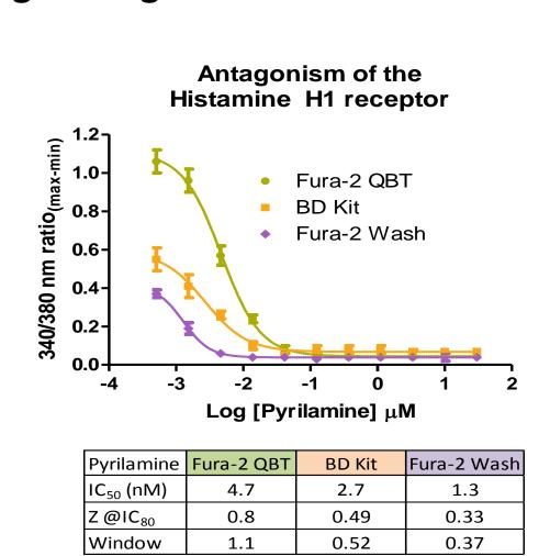
Figure 4. 7,500 cells per well were plated the same manner as the CHO-M1 cells in Figure 3 above. 2.5 mM probenecid was used to help keep the dye inside the cells. Agonist  $EC_{50}$  and antagonist  $IC_{50}$  values were within one-half log of each other as well as published values. In the pyrilamine assay, challenge agonist was 40 nM histamine. Fura-2 QBT Calcium kit had the largest signal window compared to both traditional wash assay and the BD kit.
