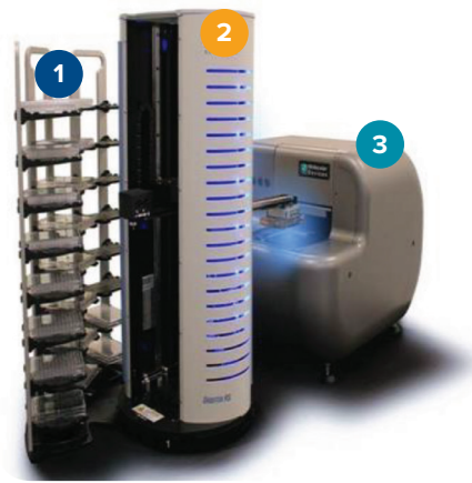
Figure 1. A typical instrument setup to achieve automated plate delivery to the cell colony imager. 1. Plate hotel. 2. Robotic arm. 3. CloneSelect Imager.
