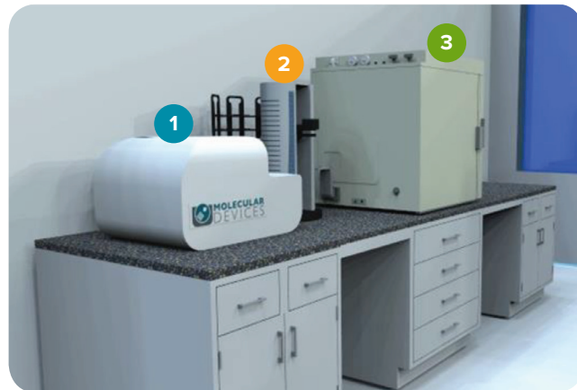
Figure 2. A typical instrument setup to achieve automated plate delivery between the cell colony imager and incubator. 1. CloneSelect Imager. 2. Robotic arm. 3. Incubator.
