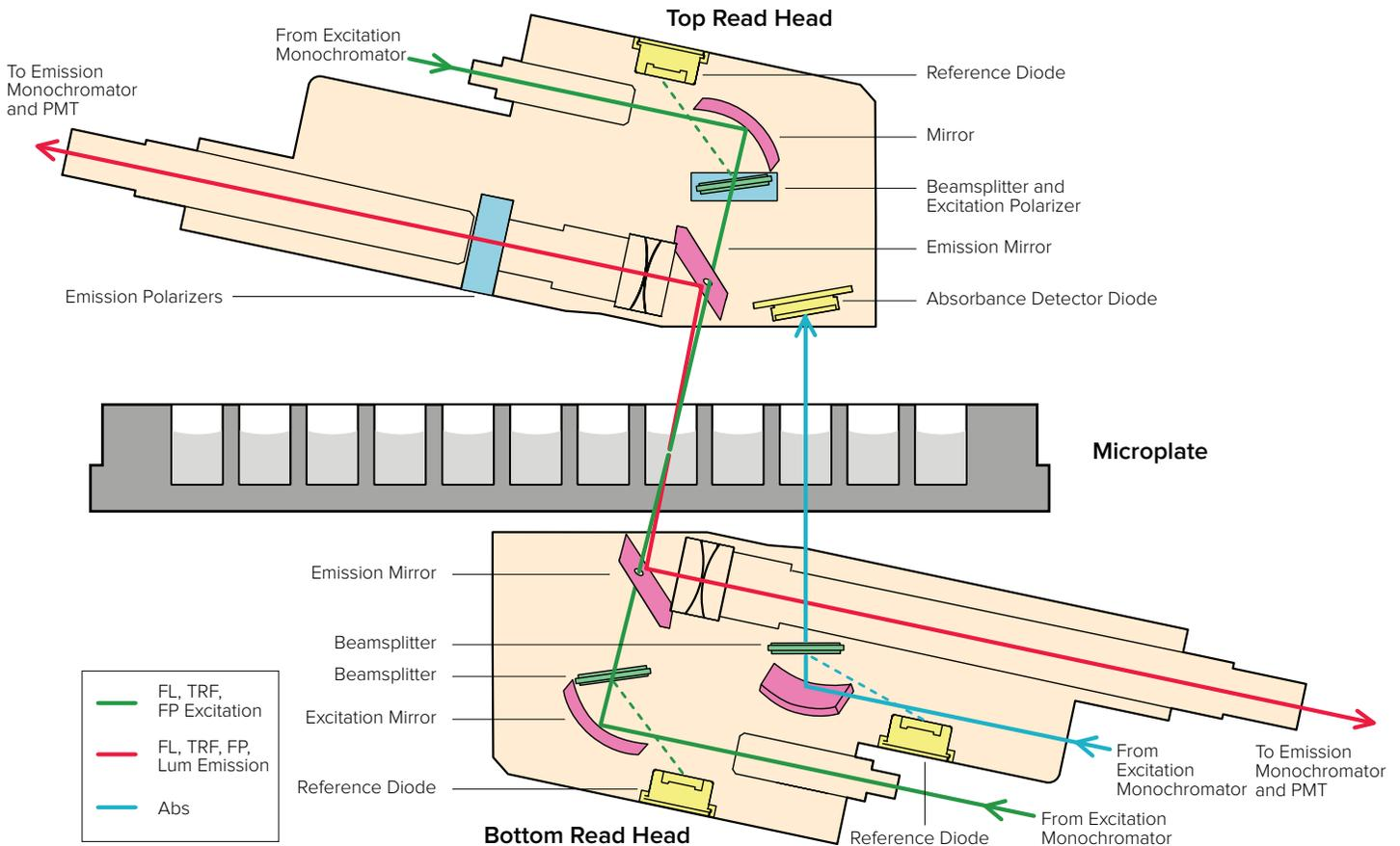
**Five-mode microplate reading with superior optics.**
